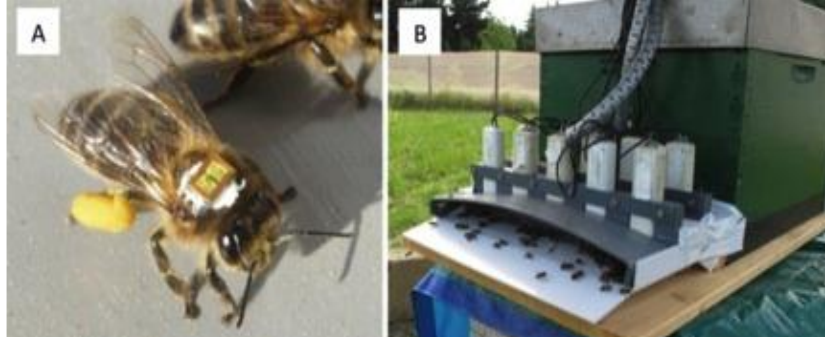
Honey bee RFID monitoring equipment. (A) A pollen-forager honey bee fitted with a 3-mg RFID tag. (B) A hive entrance equipped with RFID readers for detecting returning marked foragers (Henry et al., 2012)
